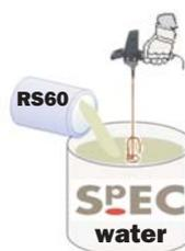
Mix in a suitable container using a trowel. As the product set time is short, only mix sufficient material which can be used in the time available.
